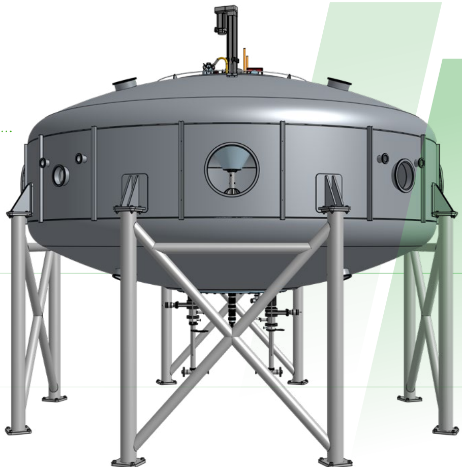
OpenStar's Vacuum Chamber designed in Onshape
