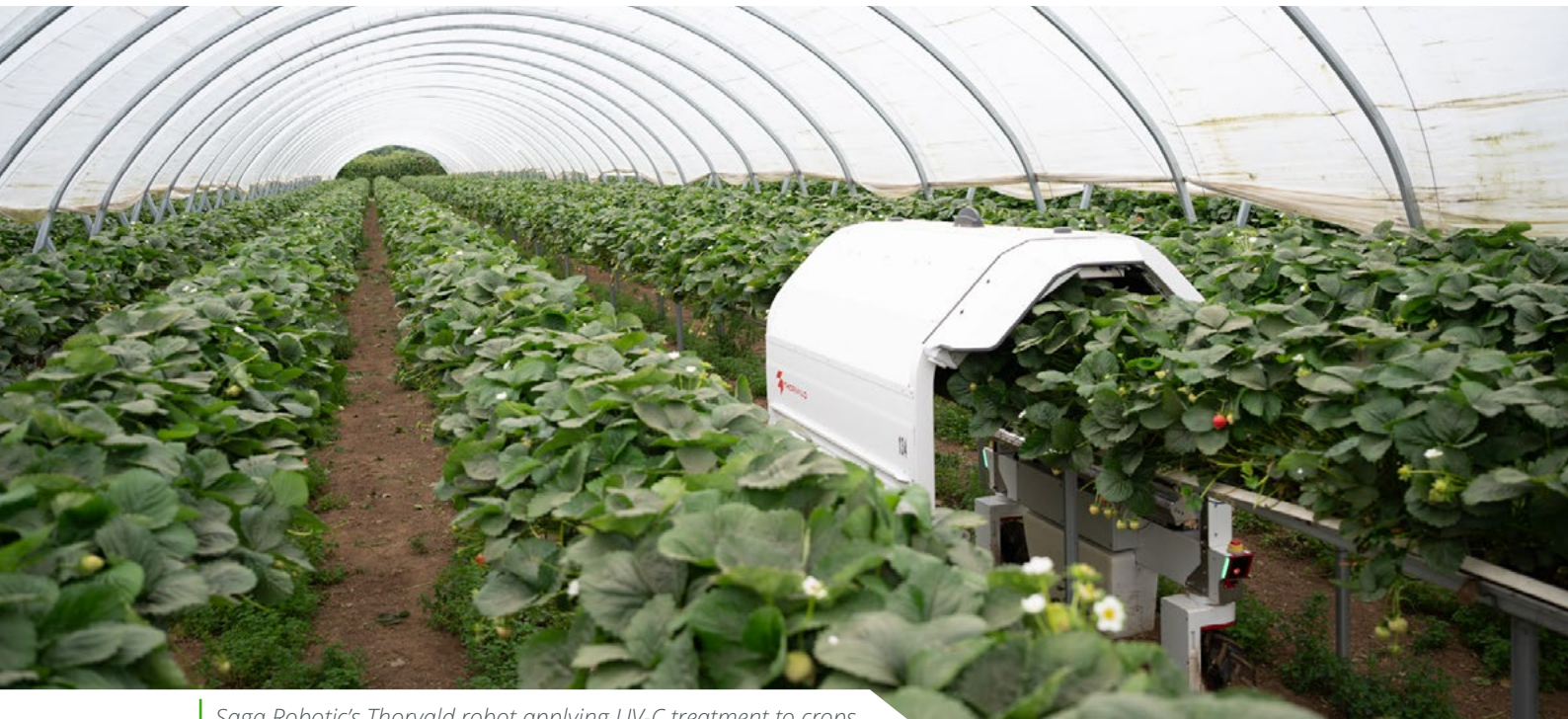
| Saga Robotics' Thorvald robot applying UV-C treatment to crops
