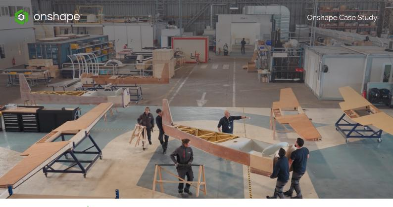
The fuselage of Aura Aero's INTEGRAL aircraft is made from a blend of wood and carbon fiber. The direction of the wood grain can determine the strength of the assembly, according to stress analysis results.
