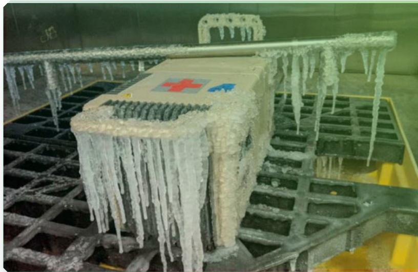
Delta Development's Autonomous Portable Refrigeration Unit (APRU) is designed to withstand both extreme hot and cold conditions.
