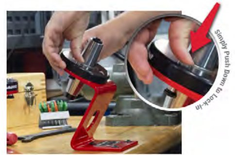
Step 2: Lock-in System + Place thumbs on both buttons. Push down to securely and accurately lock-in tool.
