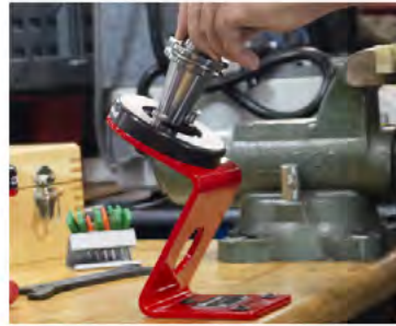
Step 1: Insert Tool + Place tooling inside tool fixture.
