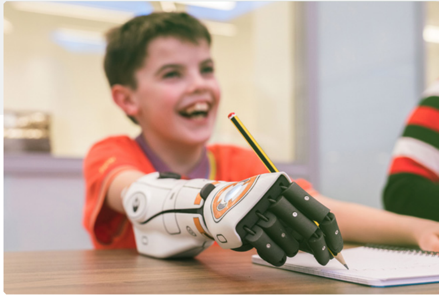
The Hero Arm, shown here with the Star Wars BB-8 magnetic cover, can be programmed with up to six easy-to-select grips to help users perform a variety of daily tasks.
